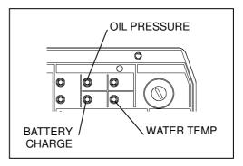
When abnormality is detected, the corresponding monitor lamp will flash, and the engine is automatically shutoff.
