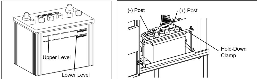
■ Replacing the Battery
