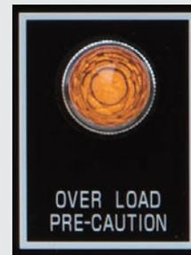
The lamp starts to flash if the output current exceeds 80% of the rated current.
