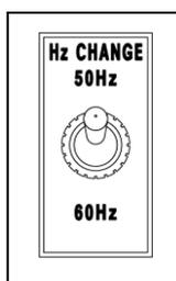
This switch functions a covert the frequency for 50Hz or 60Hz. It locates inside of the operation panel. Loosen the two screws and open the operation panel. The setting and frequency in equipment should be identical.
