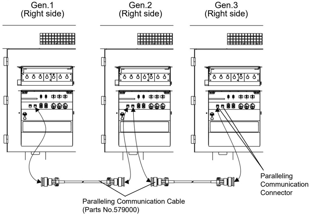
■ For three-phase load: (parallel operation)
