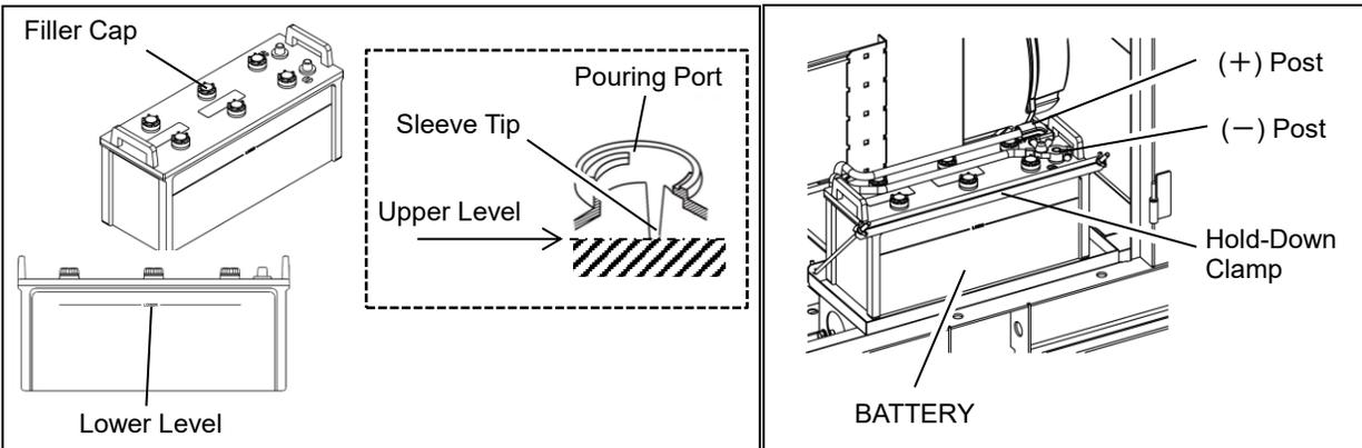
**■ Replacing the Battery**
