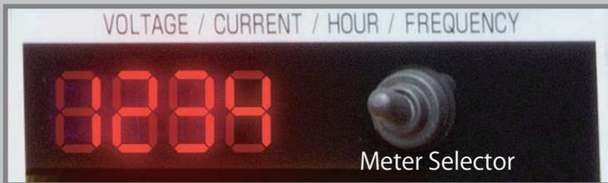
The equipment includes a meter that provides digital display or voltage, current, operating time, and frequency. Meter is equipped with meter selector that can be switched to display voltage **VOLT**, current **Curr**, operating time **Hour** or frequency **FREQ**.
