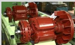
Triple-varnish, standard spec for Shindaiwa's alternator for export, offers robust features of protection against sand gravel, dust, rodent, and burnout including layer short
