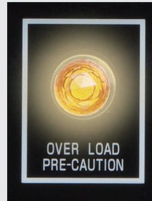
3-phase output from R, S and T terminals are monitored. When the current from either of these terminals reaches 80% of the rated output, the warning lamp starts to flash to alert it.
